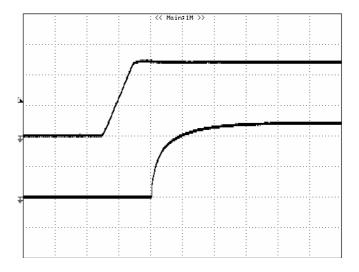
**Figure 4:** Turn-on transient at full rated load current (5ms/div). Vin=48V. Top Trace: Input Voltage, 20V/div; Bottom Trace: Vout, 5V/div
