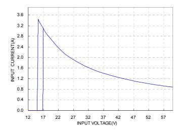
Figure 3: Typical full load input characteristics at 25°C
