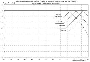
Figure 23: Output current vs. ambient temperature and air velocity @Vin=48V (Transverse orientation, airflow from Vin- to Vin+)
