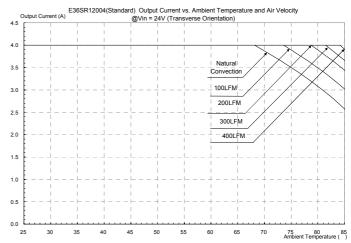
Figure 22: Output current vs. ambient temperature and air velocity @Vin=24V (Transverse orientation,airflow from Vin- to Vin+)
