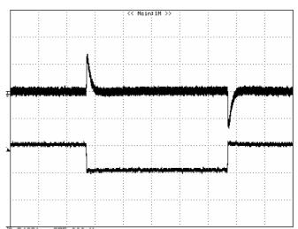
Figure 8: Output voltage response to step-change in load current (75%-50%-75% of lo, max; di/dt = 0.01A/μs). Load cap: 10μF tantalum capacitor and 1μF ceramic capacitor. Top Trace: Vout (0.1V/div, 1ms/div), Bottom Trace: lout (1A/div). Scope measurement should be made using a BNC cable (length shorter than 20 inches). Position the load between 51 mm to 76 mm (2 inches to 3 inches) from the module
