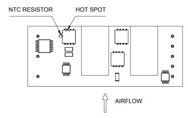
Figure 21: \* Hot spot& NTC resistor temperature measured points.
