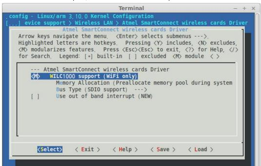
Heap area used in ATWILC1000 Driver can be chosen by user as allocation time. If system memory is shortage, choose first item.
