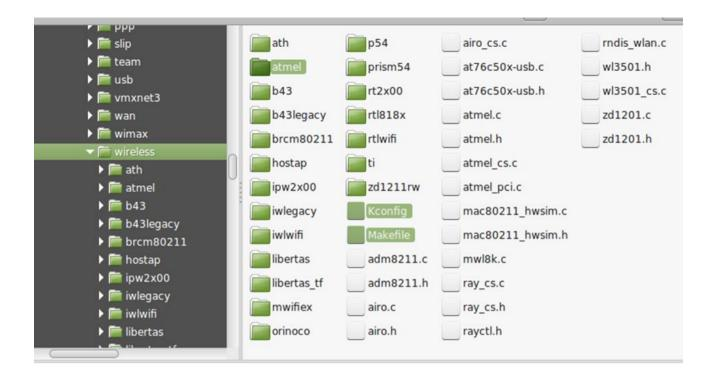
To include the ATWILC1000 driver in Kernel build, relevant Kconfig and Makefile are also changed.
