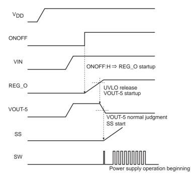
\* Be sure to set the ONOFF to 0V when starts or stops  $V_{DD}$ . And apply voltage to VIN after  $V_{DD}$  started up.
