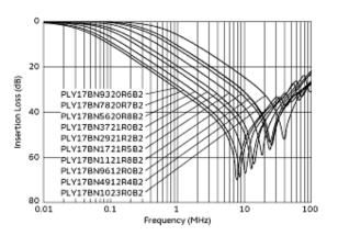
Common Mode Insertion Loss-Frequency Characteristics
