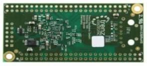
Product information "FPGA Module with Xilinx Artix-7 XC7A100T-2CSG324C, 2 x 50 Pin with 2.54 mm pitch"
