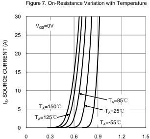
V<sub>SD</sub>, SOURCE-DRAIN VOLTAGE (V) Figure 9. Diode Forward Voltage vs. Current
