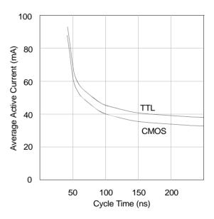
Figure 3: I<sub>CC</sub> (max) Writes
