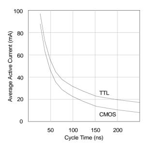
Figure 2: I<sub>CC</sub> (max) Reads
