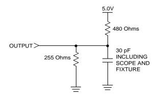
Figure 1: AC Output Loading
