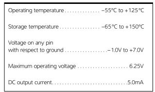
\*NOTICE: Stresses beyond those listed under "Absolute Maximum Ratings" may cause permanent damage to the device. This is a stress rating only and functional operation of the device at these or any other conditions beyond those indicated in the operational sections of this specification is not implied. Exposure to absolute maximum rating conditions for extended periods may affect device reliability.
