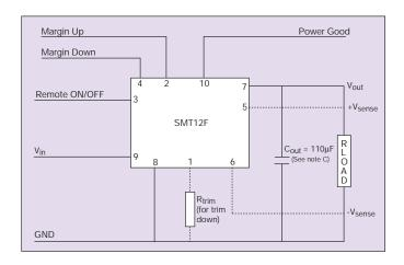
Figure 4 - Standard Application Drawing
