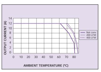
Figure 2 - Derating Curve Vin = 5 V, Output Voltage = 1.5 V (See Note A)
