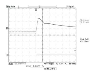
Figure 3 - Typical Transient Response (source) 12 A load Step di/dt = 300 A/μs Channel 1: Deviation on unit = 2.3%, Settling Time = 16 µs Vin = 5 V, Vout = 1.5 V
