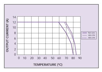
Figure 1 - Derating Curve Vin = 5 V, Output Voltage = 1.8 V (See Note A)
