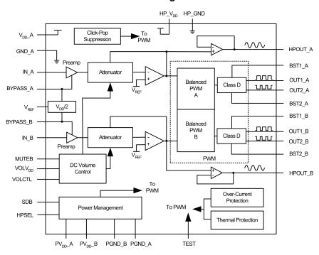
Figure 1. Block Diagram for LM4682
