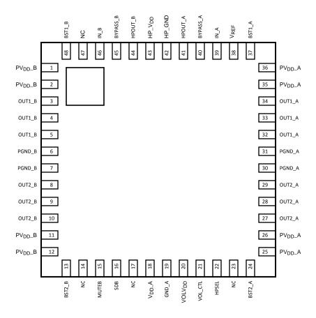
Figure 2. 48-Lead WQFN - Top View See RHS Package
