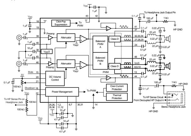
Figure 3. Typical Stereo Audio Amplifier with Headphone Selection Circuit
